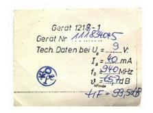
Each unit was issued with a certificate (See also Chapter 128). This 31218 certificate contain the type and serial number, DC input voltage and current, frequency, AF input sensitivity at  $\pm$  75kHz deviation and RF output into 50 $\Omega$ .
